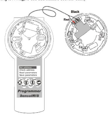
You can find a detailed connection diagram for every magpro (modules, detectors, call points or sounders) in its individual installation manual.
